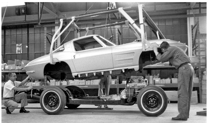
The photo at right shows the absence of a steel fuel tank in the chassis indicating the fiberglass 36.5-gallon tank is in the body. The Daytona blue car to be driven by Doug Hooper was shipped by Flying Tiger air freight to Mickey Thompson's shop in Long Beach, California on September 12, 1962 to allow the Thompson shop time to prepare the car.
